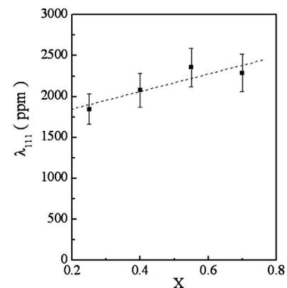
FIG. 4. Concentration dependence of the spontaneous magnetostriction  $\lambda_{111}$  of the  $\text{Dy}_{0.7-x}\text{Tb}_x\text{Pr}_{0.3}(\text{Fe}_{0.9}\text{B}_{0.1})_{1.93}$  cubic phase.
