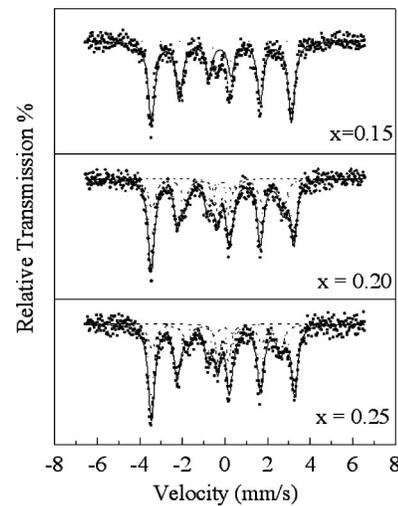
FIG. 3. Mössbauer spectra at RT for  $\text{Dy}_{0.7-x}\text{Tb}_x\text{Pr}_{0.3}(\text{Fe}_{0.9}\text{B}_{0.1})_{1.93}$  alloys.
