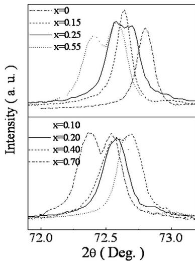
FIG. 2. Profiles of the (440) line of the  $\text{Dy}_{0.7-x}\text{Tb}_x\text{Pr}_{0.3}(\text{Fe}_{0.9}\text{B}_{0.1})_{1.93}$  cubic Laves phase.
