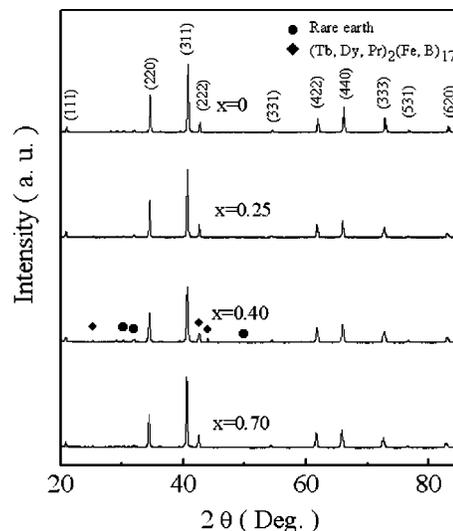
FIG. 1. XRD patterns of homogenized  $\text{Dy}_{0.7-x}\text{Tb}_x\text{Pr}_{0.3}(\text{Fe}_{0.9}\text{B}_{0.1})_{1.93}$  alloys. ( $h,k,l$ ) of the Laves phase was indexed.
