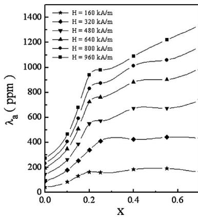
FIG. 5. Linear anisotropy magnetostriction  $\lambda_a$  at different applied fields for polycrystalline  $\text{Dy}_{0.7-x}\text{Tb}_x\text{Pr}_{0.3}(\text{Fe}_{0.9}\text{B}_{0.1})_{1.93}$  alloys at RT.
