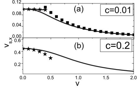
FIG. 1. Sound speed for a BEC in a 1D optical lattice via the strength of the optical lattice. The numerical results are denoted by the solid lines, analytical results for weak potentials by stars ( $\star$ ), and analytical tight-binding results by solid squares ( $\blacksquare$ ). Sound speed of  $v_{s,x}$  is in units of  $2\hbar k_L/m$ , the nonlinear coefficient  $c = \pi n_0 a_s / k_L^2$ , and the lattice strength of  $v$  is in units of  $4\hbar^2 k_L^2 / m$ .
