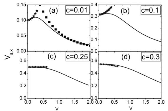
FIG. 2. Sound speed for a BEC in a 2D optical lattice via the strength of the optical lattice. The numerical results are denoted by the solid lines, analytical results for weak potentials by stars ( $\star$ ), and analytical tight-binding results by solid squares ( $\blacksquare$ ). Sound speed of  $v_{s,x}$  is in units of  $2\hbar k_L/m$ , the nonlinear coefficient  $c = \pi n_0 a_s / k_L^2$ , and the lattice strength of  $v$  is in units of  $4\hbar^2 k_L^2 / m$ .
