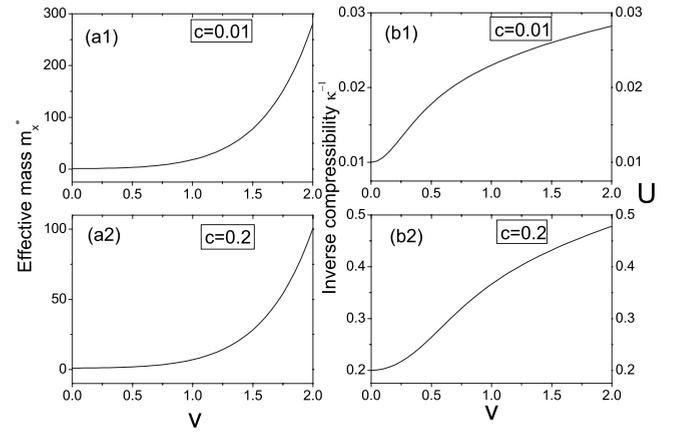
FIG. 4. Inverse compressibility  $\kappa^{-1}$  and effective mass  $m_x^*$  for a BEC in a 1D optical lattice via the strength of the optical lattice. Based on Eq. (38),  $U$  is equal to  $\kappa^{-1}$  in the tight-binding limit. The nonlinear coefficient  $c = \pi n_0 a_s/k_L^2$ , inverse compressibility  $\kappa^{-1}$  and  $U$  are in units of  $4\hbar^2 k_L^2/m$ , and the lattice strength  $v$  is in units of  $4\hbar^2 k_L^2/m$ .
