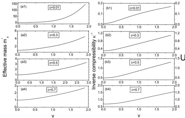
FIG. 6. Inverse compressibility  $\kappa^{-1}$  and effective mass  $m_x^*$  for a BEC in a 3D optical lattice via the strength of the optical lattice. Based on Eq. (38),  $U$  is equal to  $\kappa^{-1}$  in the tight-binding limit. The nonlinear coefficient  $c = \pi n_0 a_s / k_L^2$ , inverse compressibility  $\kappa^{-1}$  and  $U$  are in units of  $4\hbar^2 k_L^2 / m$ , and the lattice strength  $v$  is in units of  $4\hbar^2 k_L^2 / m$ .
