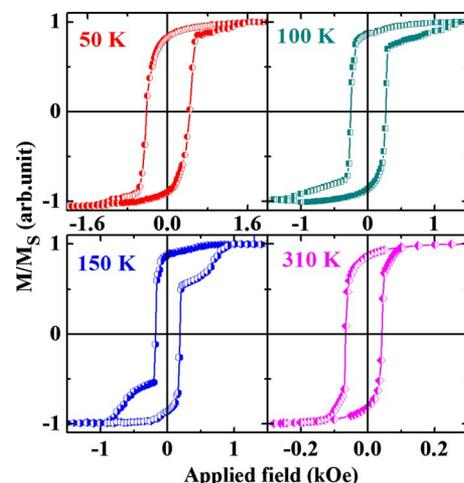
FIG. 1. (Color online) Hysteresis loops at 50, 100, 150, and 310 K of Co(3 nm)/NiO(6 nm)/Fe(10 nm) after ZFC.
