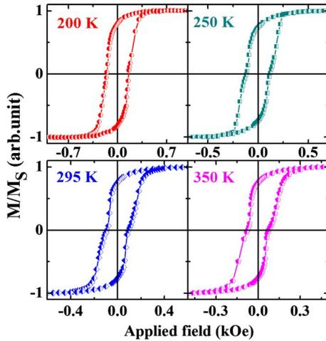
FIG. 2. (Color online) Hysteresis loops at 200, 250, 295, and 350 K of Co(3 nm)/Cr(6 nm)/Fe(10 nm) after ZFC.
