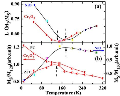
FIG. 4. (Color online) (a) Temperature dependence of  $L$  of Co(3 nm)/NiO(6 nm)/Fe(10 nm) and Co(3 nm)/Cr<sub>2</sub>O<sub>3</sub>(6 nm)/Fe(10 nm) after ZFC. (b) Temperature dependence of  $M_S/M_{120}$  for Co(3 nm)/Cr<sub>2</sub>O<sub>3</sub>(6 nm)/Fe(10 nm) after ZFC and FC, and  $M_S/M_{150}$  for Co(3 nm)/NiO(6 nm)/Fe(10 nm) after ZFC.
